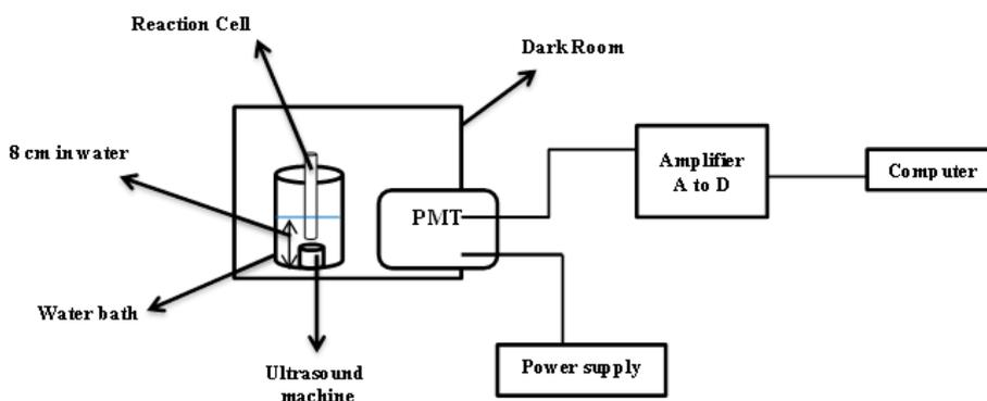
Figure 2. Block diagram of Sonochemiluminescence instrument
