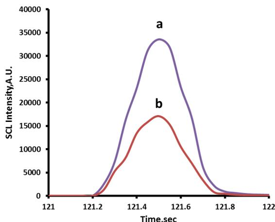
Figure 4. Effect of penconazole on SCL of luminol. a: Blank. b: Penconazole  $1.0 \times 10^{-3}$
